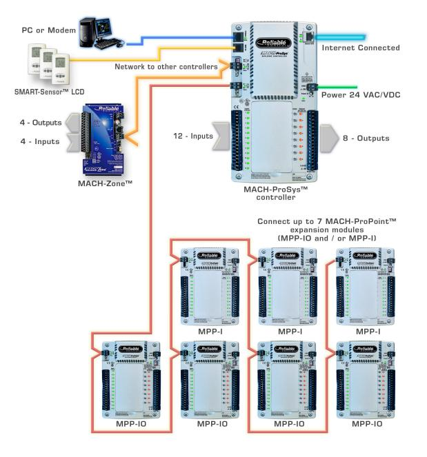
Connect up to 7 MACH-ProPoint<sup>™</sup> expansion modules (MPP-IO and MPP-I) with a maximum possible input count of 128, a maximum possible output count of 64, and a maximum total I/O of 160 per controller.
