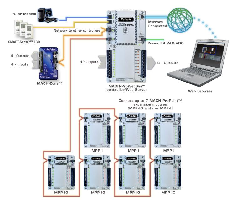
Connect up to 7 MACH-ProPoint<sup> $\infty$ </sup> expansion modules (MPP-IO and MPP-I) with a maximum possible input count of 128, a maximum possible output count of 64, and a maximum total I/O of 160 per controller.
