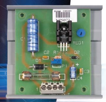
The Reliable Controls® PS-VDC is a robust, low-cost variable DC power supply for energizing building automation peripheral devices.
