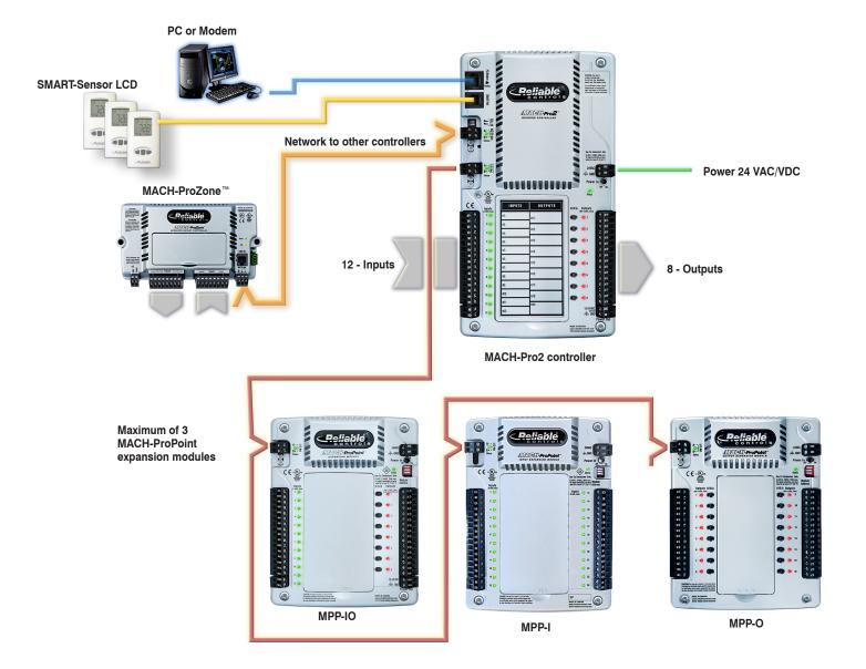
Connect up to 3 MACH-ProPoint expansion modules (MPP-I, MPP-IO, MPP-IO-U and/or MPP-O) with a maximum input count of 84, and a maximum output count of 56 per controller. Expansion modules are daisy-chained to the I/O-Net port of a MACH-Pro2 controller in any combination while limiting the total inputs, outputs, and modules below maximum.
